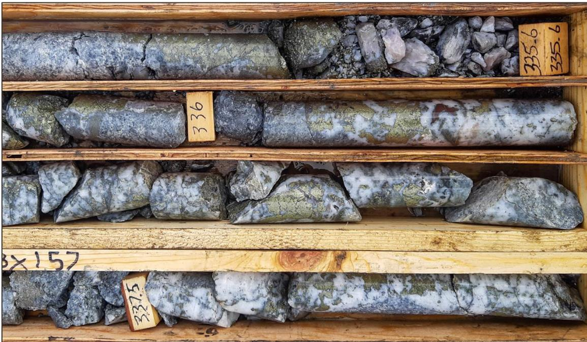
**Plate 7.7 JT Deposit – Footwall Copper Zone (FWCZ) in Hole JT19-089**
