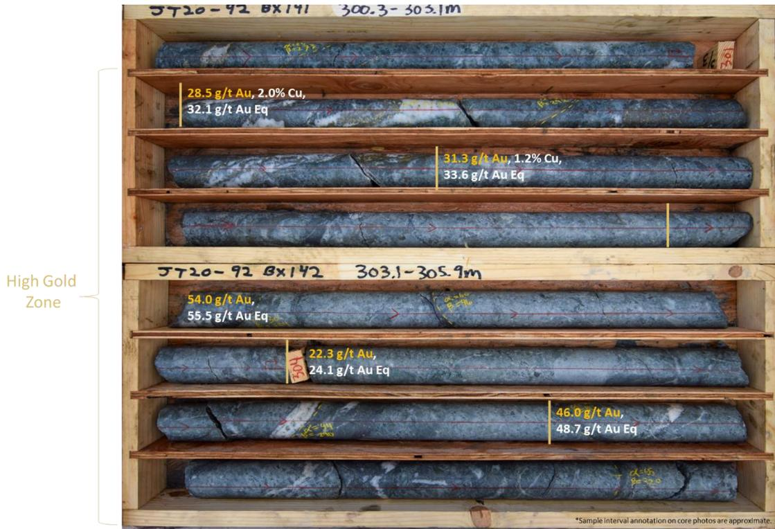
**Plate 7.4 JT Deposit – Example of Mineralized Drill Core from Hole JT20-92**
