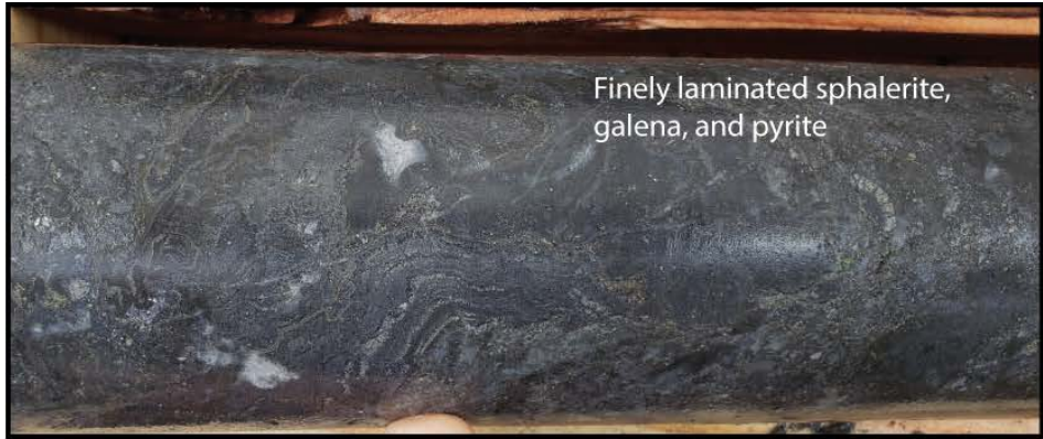
Plate 1. Core photos of VMS-style mineralization from drillhole JT20-114
